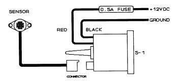
All wiring connections shall be made using #16 Gauge stranded copper wire conforming to ABYC standards for marine use.
